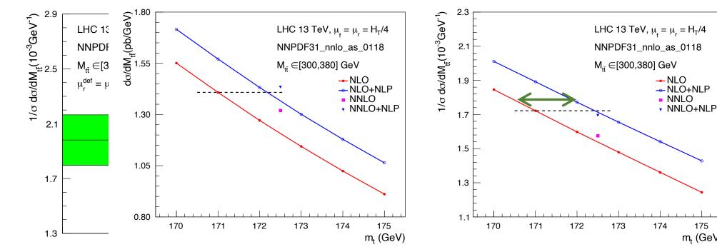
The prediction for  $m_t = 172.5 \text{ GeV}/c^2$  moves towards the CMS measurements when including Coulomb corrections.
