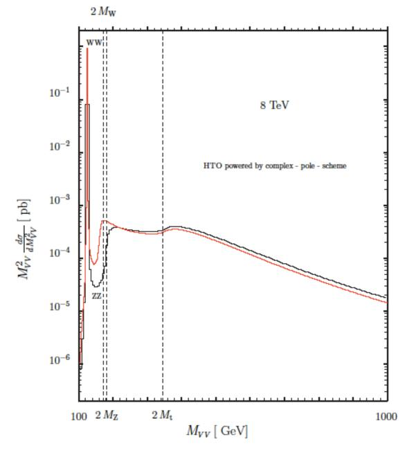
Figure 2. The NNLO ZZ (black) and WW (red) invariant mass distributions in  $gg \to VV$  for  $\mu_H = 125\,\text{GeV}$ .
