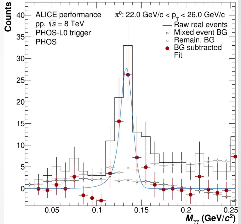
Photon Conversion Method (PCM) uses tracking detectors and provides excellent accuracy at low  $p_T$ , electromagnetic calorimeters PHOS has good resolution at high  $p_T$ .
