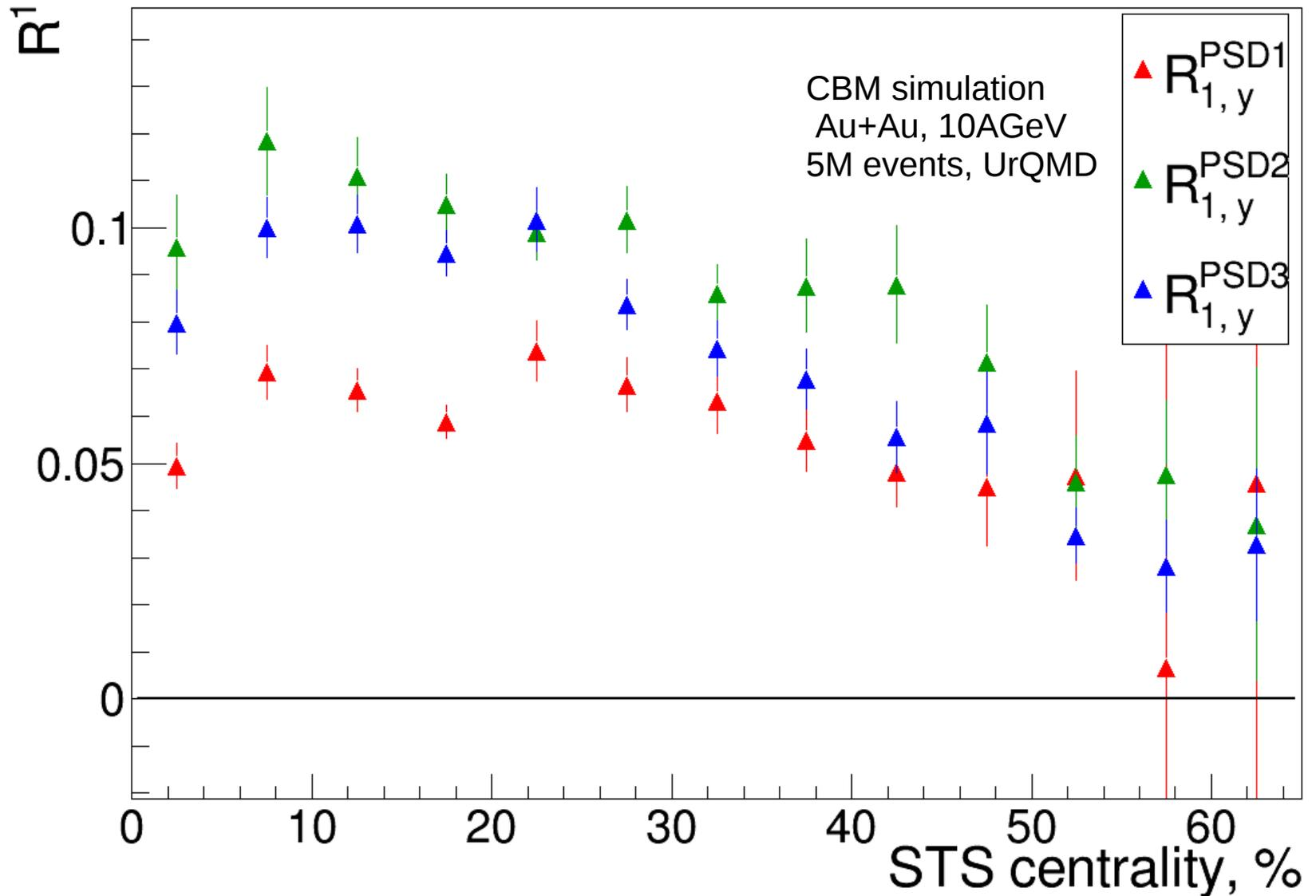
Central part has worse resolution. Can be improved with higher granularity
