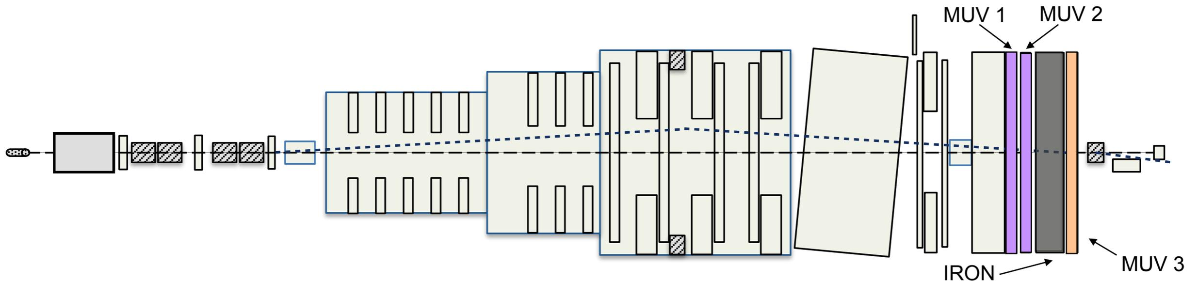
**MUV 3:** Efficient fast Muon Veto used in the hardware trigger level.
