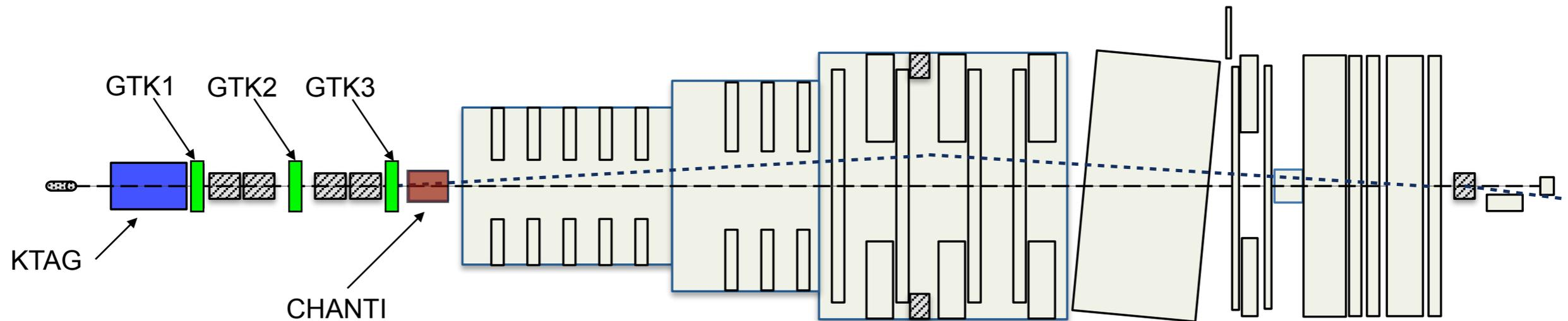
**KTAG** is an upgrade of CERN Cedar: Čerenkov Differential counter with Achromatic Ring focus blind to all particles but kaons of appropriate momentum (75 GeV, K<sup>+</sup> rate:~45MHz).
