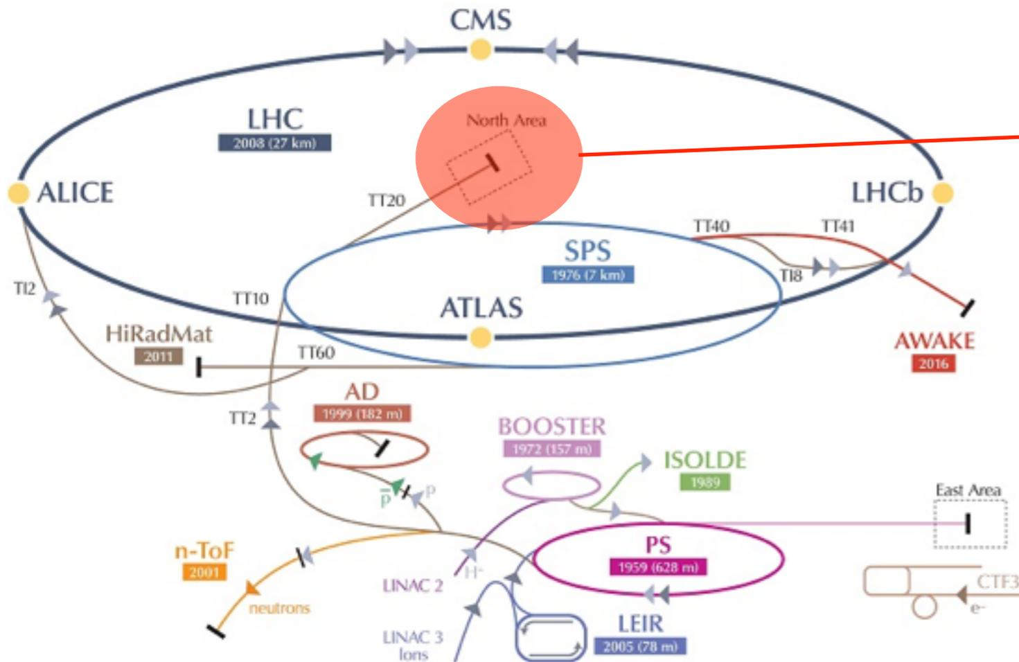
NA62 is housed in the CERN North Area. The SpS extraction line is providing a secondary charged hadron beam 50 times more intense than in the past, with only 30% more SPS protons on target.
