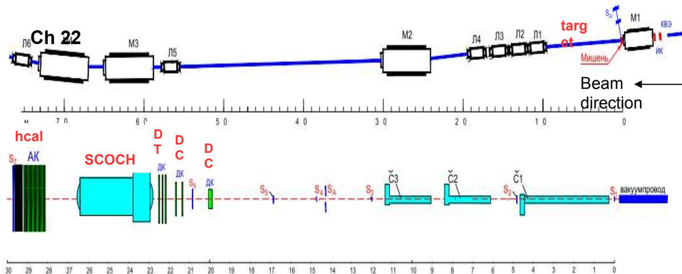
*Si*-scintillation counters, *Ч* - Cherenkov counters, *SCOCH* – RICH detector, *hcal* - hadron calorimeter, *DT* – drift tubes, *DC* – drift chambers.
