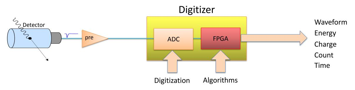
The aim of the Digital Pulse Processing is to make a "all in digital" version of analog modules such as Shaping Amplifiers, Discriminators, QDCs, Peak Sensing ADCs, TDCs, Scalers, Coincidence Units, etc.
