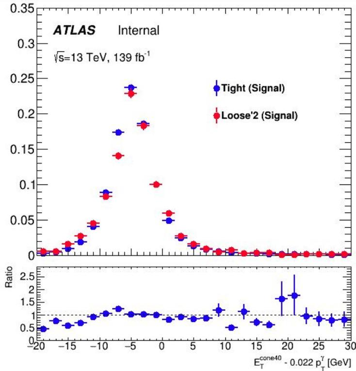
The bottom panel shows the ratio of tight photon candidates from Z+jets simulation and anti-tight photon candidates in data to the anti-tight photon candidates from Z+jets simulation.
