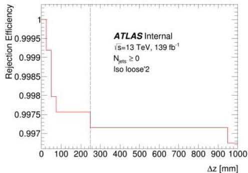
Absolute value of z coordinate pointed by the photon candidate with respect to the identified primary vertex is required to be **less than 250 mm**
