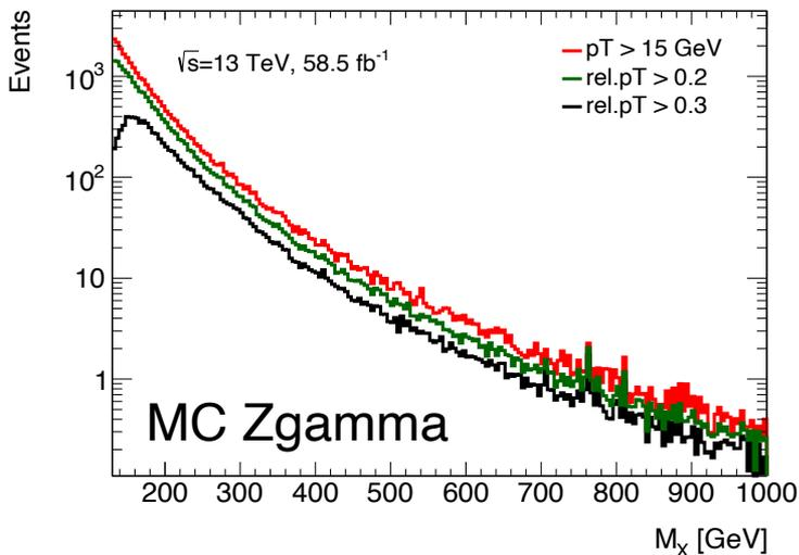
peak of signal distribution is moving with higher mass, while for background is  $\sim$ same  $\Rightarrow$  cut at 0.3 cuts more events at low masses than at high masses
