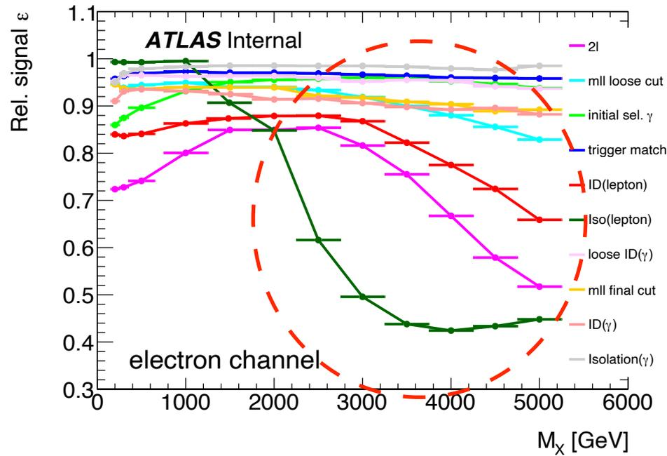
Drop of signal efficiency at high mass ( $> 1$  TeV) due to electron being highly collimated (boost effect):
