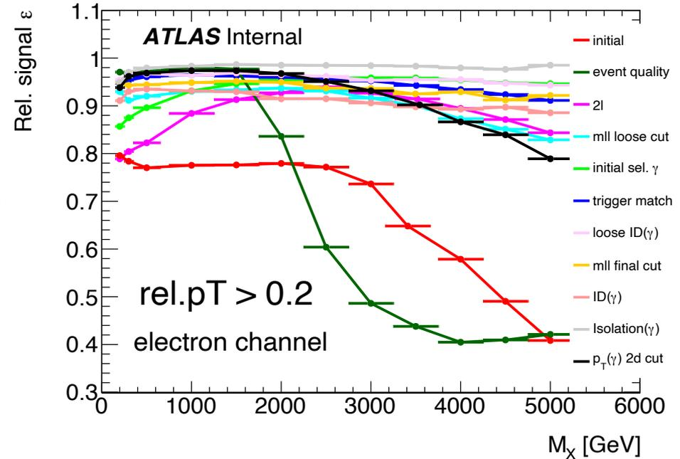
differences in lepton (pink curve) efficiency are caused by ID&Isolation cuts applied at later stages
