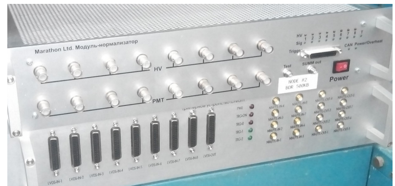
Custom built FPGA-based trigger unit hardware for iDream experiment.
