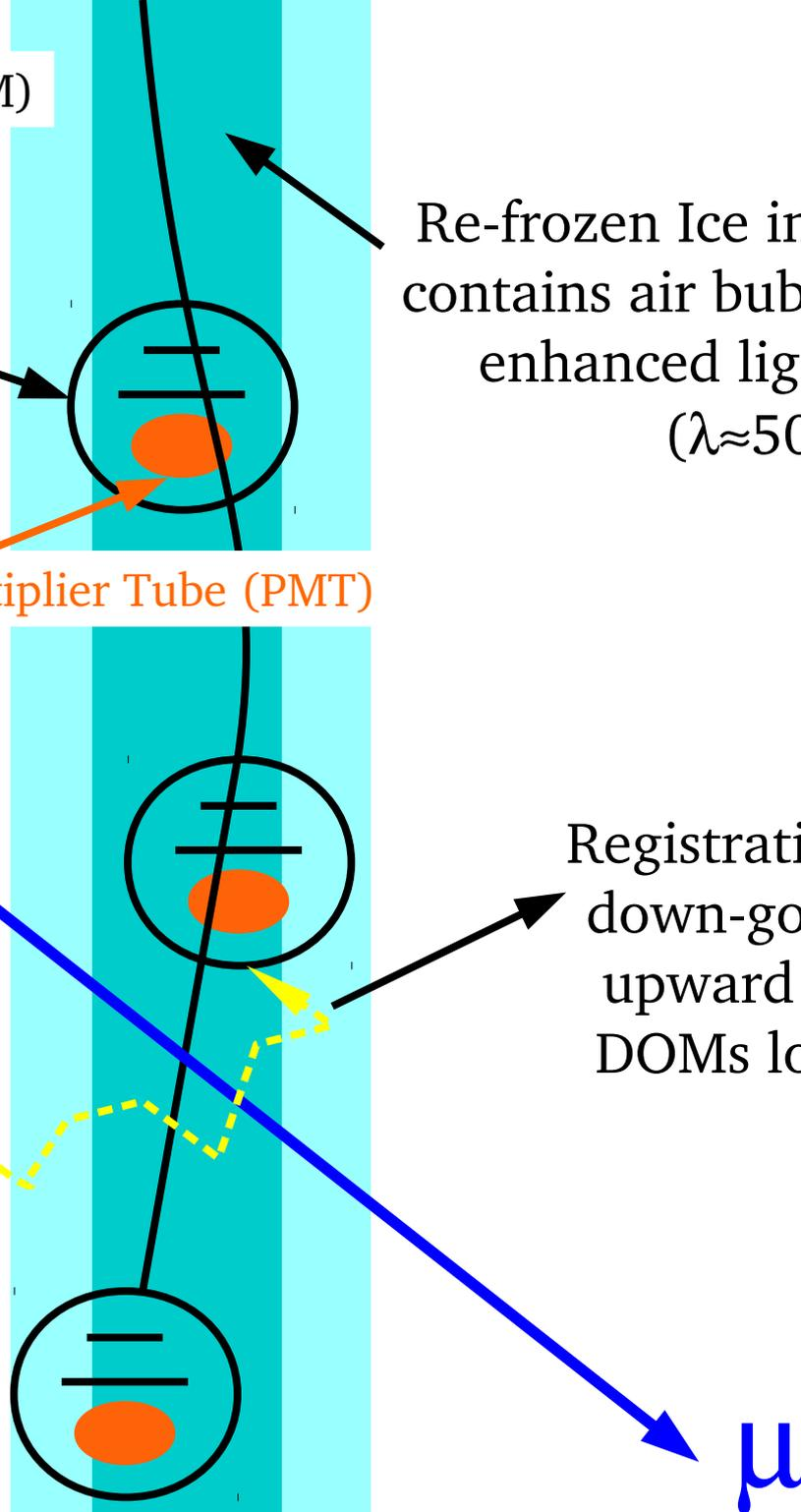
Registration of photon from down-going track requires upward scattering due to DOMs looking downward
