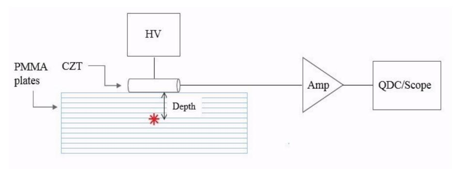
Detector (CZT) is biased through a preamplifier with +350V from a high voltage power supply (HV). Signal from the detector preamplifier is shaped and amplified with a spectrometric amplifier (Amp), and then passed to the input of Lecroy Waverunner oscilloscope, which can be used as a charge-to-digital converter (QDC/Scope).
