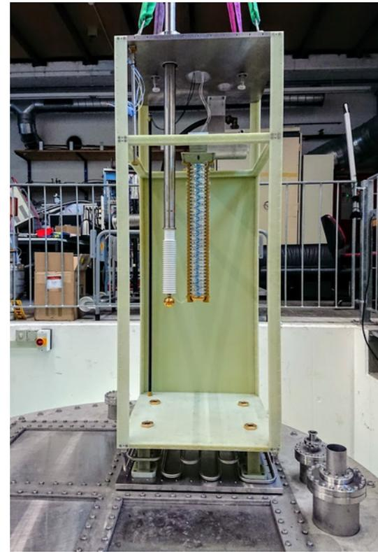
Furthermore: Test Scalability of Resistive Shell to larger drift volumes
