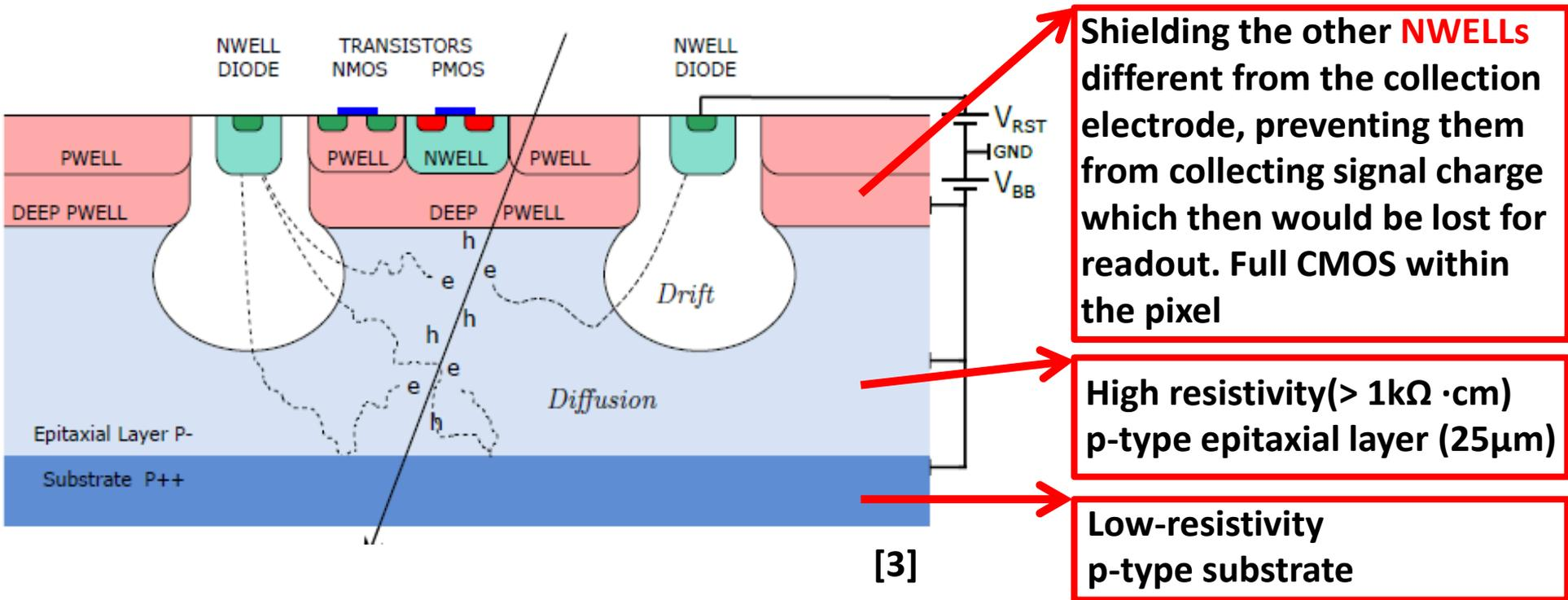
Small n-well diode (2-3 µm diameter), ~100 times smaller than pixel → low capacitance [4]
