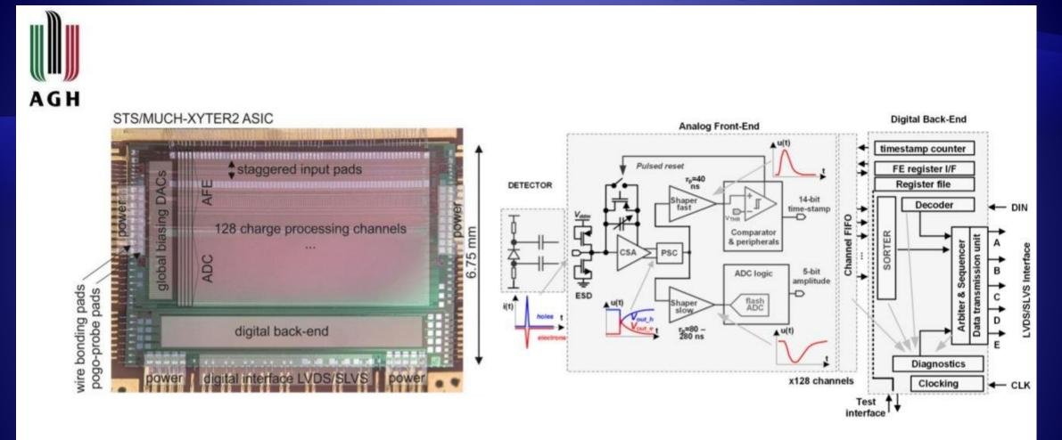
128 channels + 2 test channels
