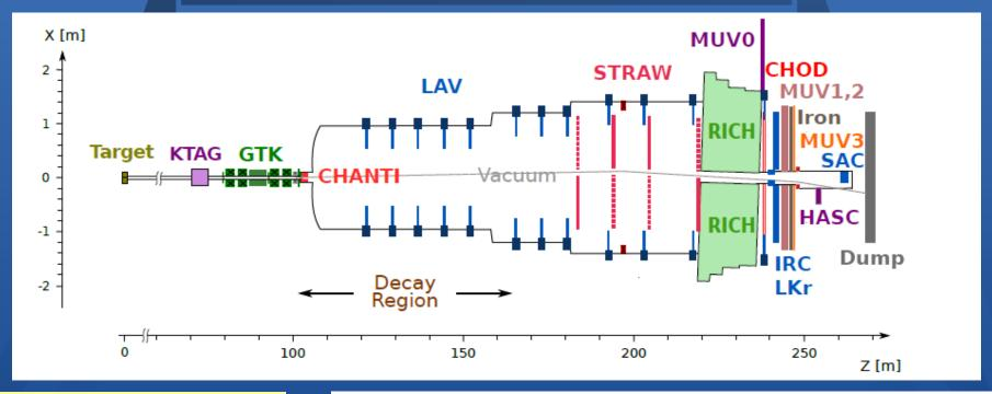
Un-separated hadron (p/π<sup>+</sup>/K<sup>+</sup>) beam. SPS protons: 400 GeV, 3×10<sup>12</sup>/spill. K<sup>+</sup>: 75GeV/c (±1%), divergence < 100μrad. 800 MHz beam rate; 45 MHz K<sup>+</sup> rate; ~5 MHz K<sup>+</sup> decays in fiducial volume Timing between sub-detectors O(100 ps).
