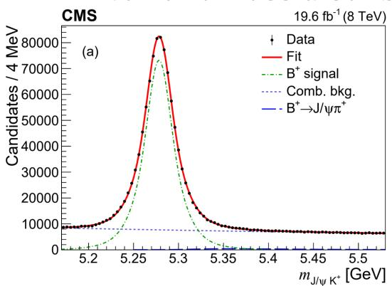
Modelled with triple Gaussian function with common mean for signal, exponential for bkg additional small contribution to account for Cabibbo suppressed  $B^+ \rightarrow J/\psi \pi^+$  decay
