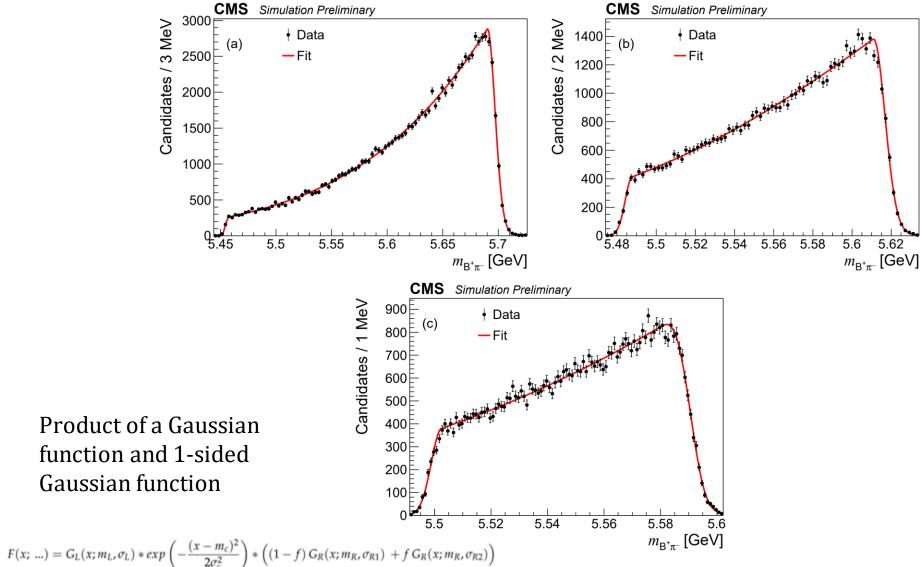
$$F(x; ...) = G_L(x; m_L, \sigma_L) * exp\left(-\frac{(x - m_c)^2}{2\sigma_c^2}\right) * \left((1 - f) G_R(x; m_R, \sigma_{R1}) + \frac{1}{2} G_R(x; m_R, \sigma_{R1})\right)$$
