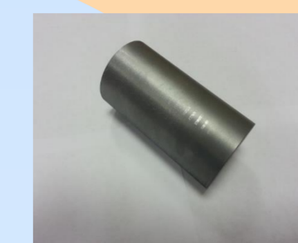
Chromium bar after HIP and mechanical operation
