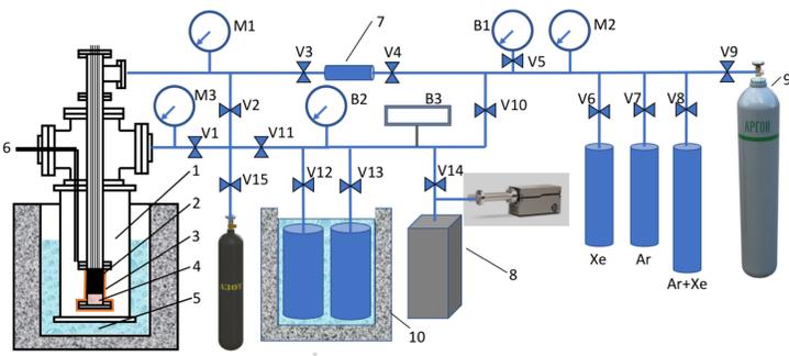
1 – vacuum vessel, 2 – PMT, 3 – copper housing, 4 – LAr volume, 5 – LN<sub>2</sub> bath, 6 – heater & thermocontrol, 7 – gas filter Mycrolys, 8 – magnetoelectrical pump Nord & RGA, 9 – Ar (purity 99,9995%), 10 – cryogenic pump; B1– B3 – vacuummeters; M1 – M3 – manometers; V1– V15 – valve.
