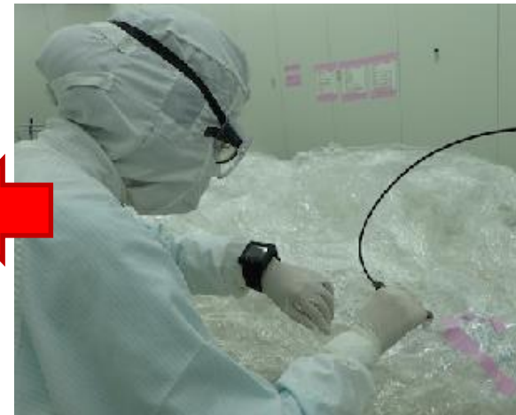
He leak check & repairing
