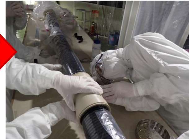
Mini-balloon parts assembling
