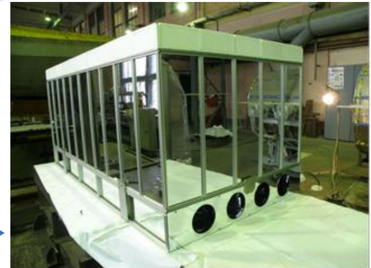
Liquid scintillator detector 50 sections 0.235x0.235x0.85m 3
