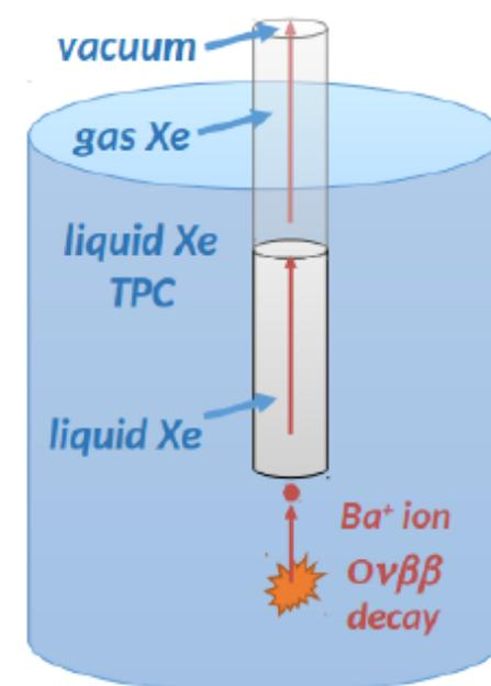
$Ba^+$  "sucked" out of LXe through capillary into ion trap and identified laser fluorescence and MRTOF spectroscopy
