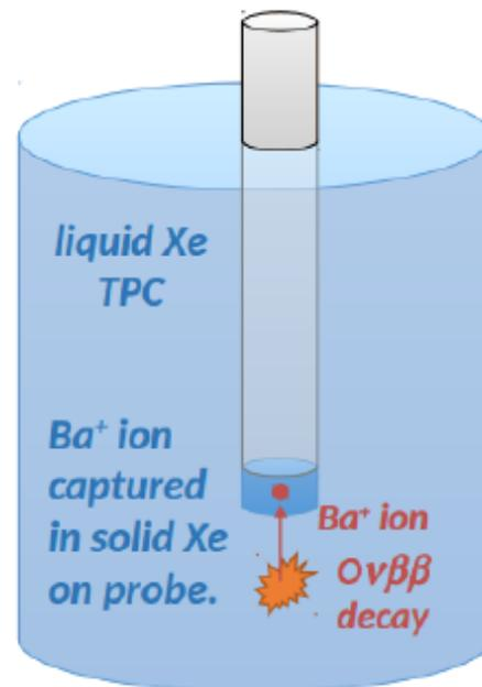
Probe removed to vacuum;  $Ba/Ba^+$  identified laser fluorescence single atom imaging in SXe
