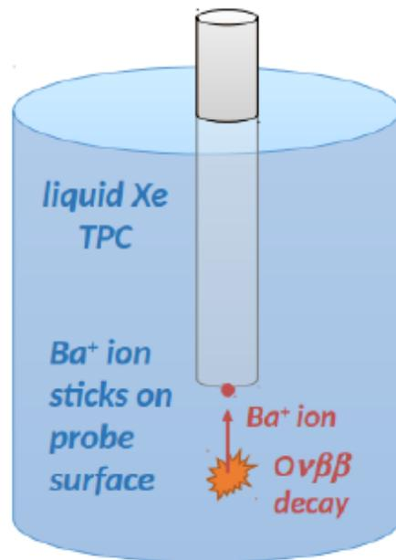
Probe removed to vacuum;  $Ba^+$  identified by (1) laser ablation/resonance ionization or (2) thermal desorption/ionization
