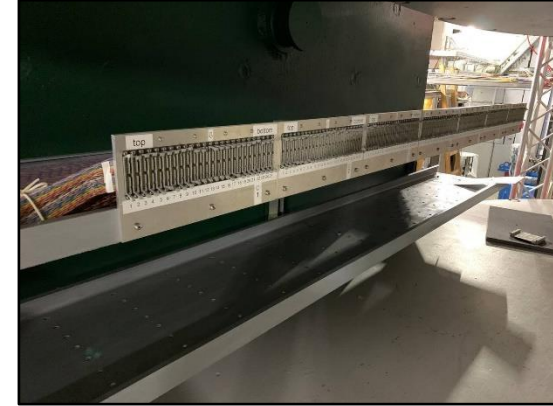
ADC cables: to patch panels↑; to DAQ rack↓
