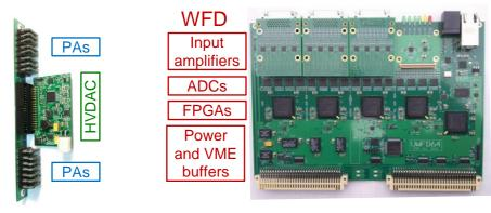
Preamplifiers PA in groups of 15 and SiPM power supplies HVDAC for each group inside shielding, current and temperature sensing
