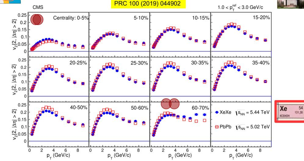
The magnitude of the v<sub>2</sub> coefficients for Xe+Xe collisions are larger than those found in Pb+Pb collisions for the most central collisions. This is attributed to a larger fluctuation component in the lighter colliding system.
