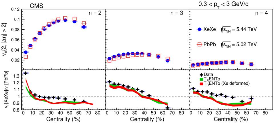
Hydrodynamic models that consider the Xe nuclear deformation are able to better describe the  $v_2[XeXe]/v_2[PbPb]$  ratio in central collisions than those assuming a spherical Xe shape.
