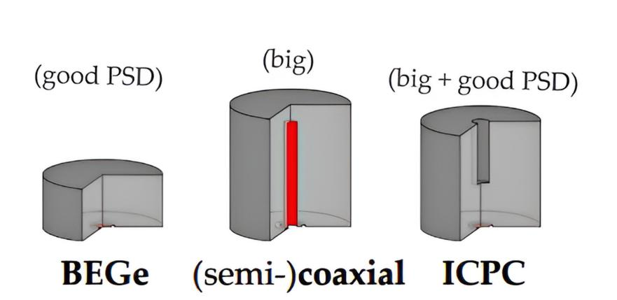
level > 90% is possible. The innovative Inverted Coaxial Point Contact (ICPC) will be one of the main detector geometries used for LEGEND since they possess a larger mass (> 2 kg) than previous point contact while still preserving good energy resolution.
