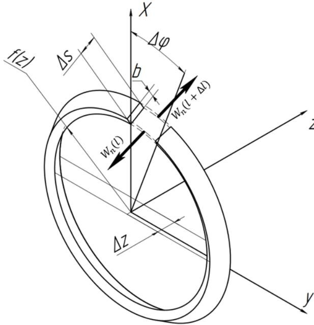
$$f(s) \frac{\partial U(s, t)}{\partial t} = \gamma \frac{\partial \left[ f(s) \frac{\partial U(s, t)}{\partial s} \right]}{\partial s} + h \delta(s)$$
