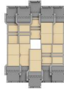
Station 2: 10 modules of 63x126 mm 2
