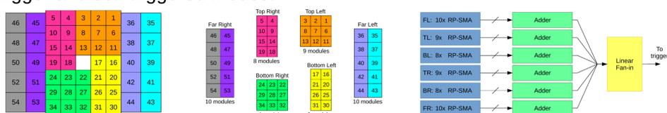
Custom 12 channel analog sum modules with adjustable attenuation for every channel were produced at JINR, Dubna. These modules were used to produce the sum of all signals in central part of the FHCAL consisting of 34 smaller modules. This signal was then used to trigger synchronous data readout from 8 ADC64 units.
