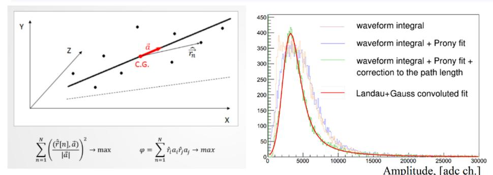
Least squares method[4] was used for track reconstruction. First, the center of gravity of deposited energy in the sections of the calorimeter is found. Then a quadratic form  $\varphi$  on a unit vector  $\vec{a}$  is maximized to find an eigenvector corresponding to a maximum eigenvalue. This vector provides the track direction. After that signal amplitudes from the track hits are corrected to the known track lengths in the scintillator tiles of the calorimeter sections.
