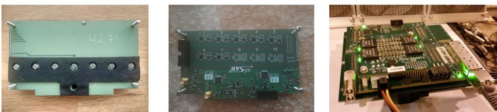
Data acquisition is performed by eight ADC64s2[2] units manufactured at JINR, Dubna. This model of 64 channel 62.5 MS/s 12-bit sampling ADCs was previously used for ZDC signal readout and therefore can be easily integrated into BM@N data acquisition system. ADC64s2 units are capable of time synchronization via White Rabbit network and can function both in external trigger and self-triggered modes.
