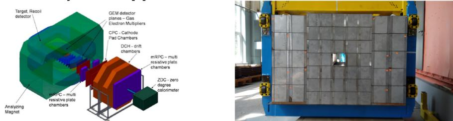
FHCAL (Forward Hadron Calorimeter) was assembled and installed at BM@N in 2019. Like ZDC in previous runs, it will be used for event plane and centrality determination. It consists of 54 lead-scintillator modules with a 15 cm by 15 cm square beam hole and is mounted on a moving platform in place of ZDC.
