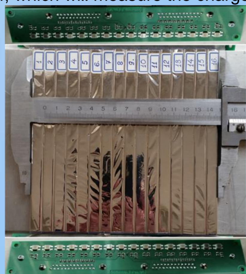
Photo of the front hodoscope during the assembly.
