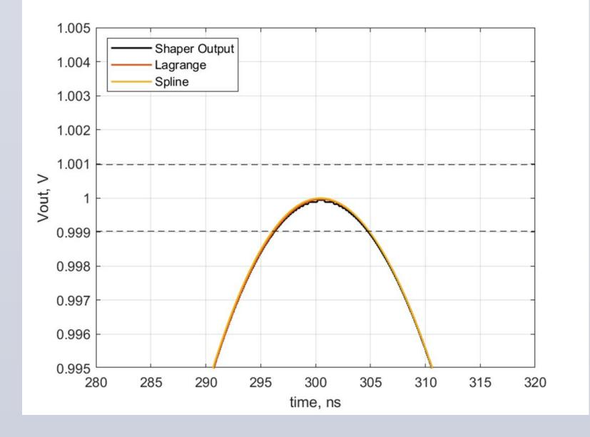
the peak without using the interpolator is 6.1 LSB, whereas with the interpolator – 1.1 LSB.
