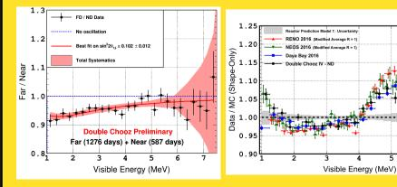
Inter-detector ratio doesn't show any spectral distortion in the 5 MeV region, thus ensuring the  $\theta_{13}$  accuracy.
