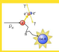
The inverse beta-decay reaction (IBD) is the corner stone in reactor neutrino physics. The IBD reaction provides specific coincidence signature: • Prompt event - positron annihilation  $E_e \approx E_v - 0.78$  MeV • Delayed event – neutron capture on all available nuclei (Gd, H,C) TnC special feature.
