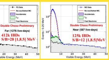
**Differences in the** accidental rate observed between FD and ND come from the fact that there is no Light Noise (LN) in ND. LN is caused by spontaneous light emission from the bases of the PMTs installed in ID.
