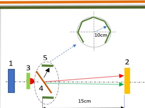
Fig. 11. Lay-out of the experimental setup. 1 – PIN-diode; 2 – Timepix3 device; 3- Cf source; 4 – thin foil (Al); 5 – PIN diodes ring. View of the ring directed at the FF beam in the insert above. For CCT mode Sn-Ni-Ca (as an example) FF velocity vectors are showed with arrows: red – Ni, green – Ca, black – Al scattered at large angle. Heavy fragment, Sn ion, hits the PIN diode (1) that is close to the source.
