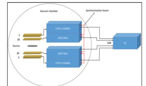
Fig.12. Schematic layout of the experimental setup for simultaneous measuring of the particle energy E by Timepix detectors and specific ionization losses  $\Delta E$  with the help of a totally depleted transmission type silicon detectors [5].
