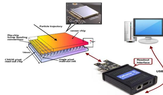
Fig. 7. Timepix3 Detector with readout device
