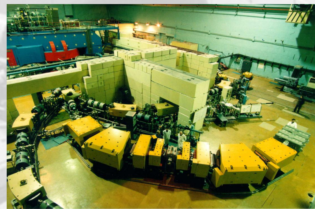
Fig.2. View of the separator COMBAS in the experimental hall of the cyclotron U-400M (beam direction from the left to the right)
