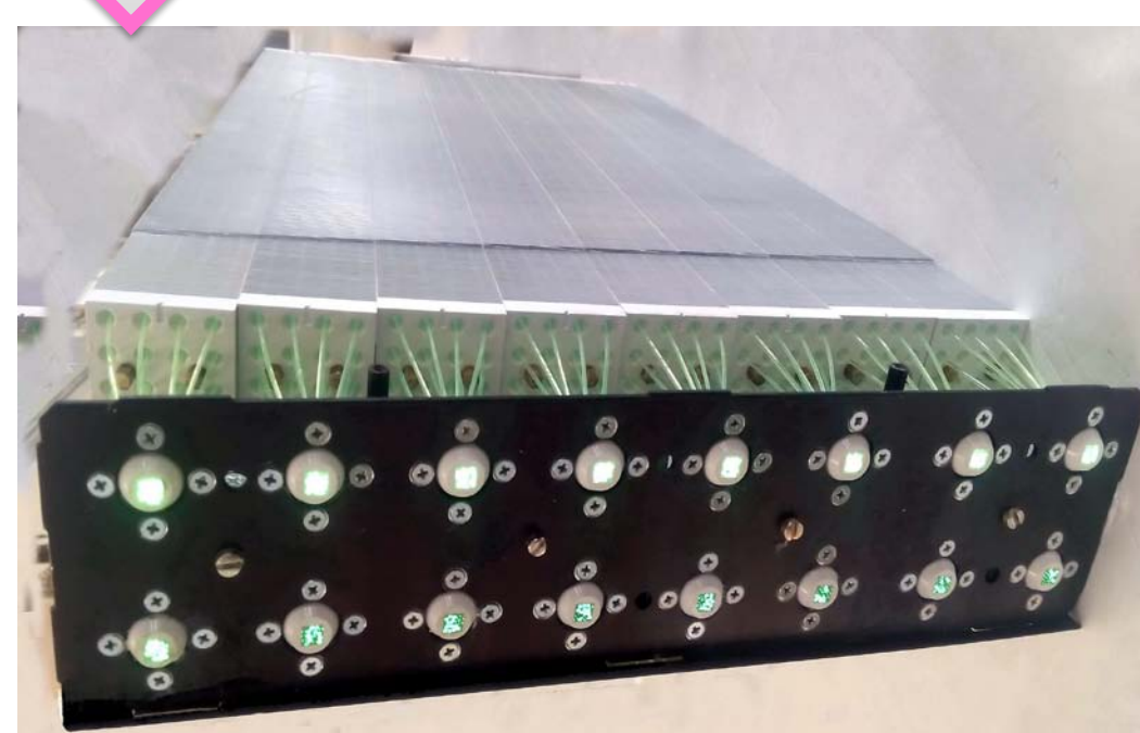
One of the first mass production ECal modules (16 towers)
