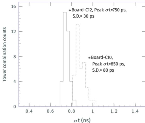
' $\sigma t$ ' is extracted from distributions of multiple combinations of any two towers.
