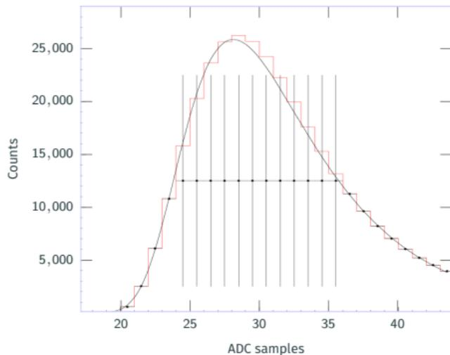
\*Considering different levels of cut on waveforms, resolution obtained after reconstructing remaining signal and integrating the signal (upper right)
