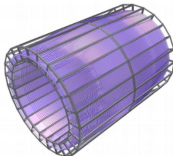
Various types of towers in all modules and sectors by their XYZ position and orientations placed together give the ECal a barrel shape
