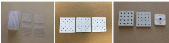
Lead, Scintillator and support plates
