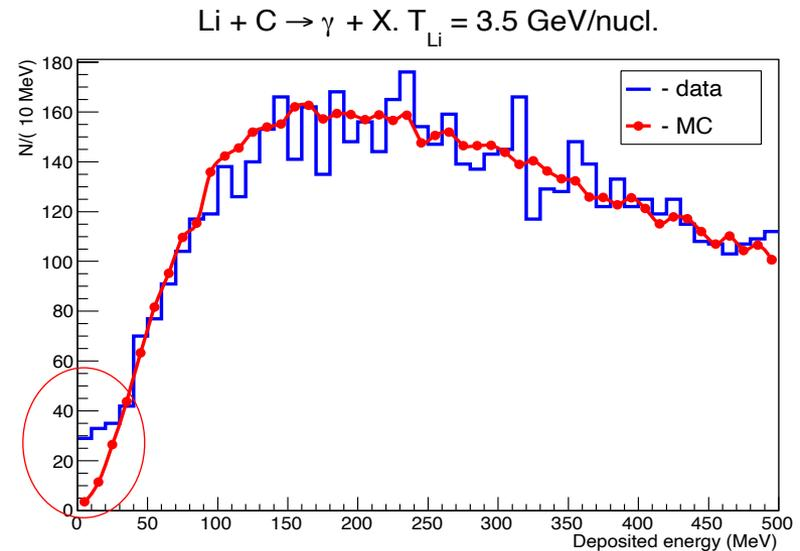
Data and **MC** spectra of energy release in ECal (BGO) & a pre-shower with 3.5 A GeV/c d and Li beams, 50<sup>th</sup>, 51<sup>st</sup> runs, Nuclotron (**SVD-2 Collaboration**)
