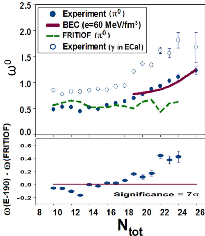
Our SVD-2 setup allows to register photons. Using original method, we have retrieved the number of events with a certain multiplicity of  $\pi^0$ 's for given  $N_{ch}$ . We've shown the ratio  $\omega^0(\text{exp})/\omega^0(\text{MC})$  gets **7s.d.** at  $N_{tot} \sim 25$  (SVD Coll., 2012).
