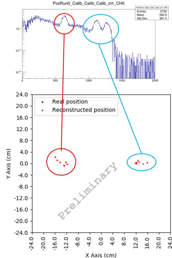
The two sources was reconstructed using the spectrum information and spatial separated.
