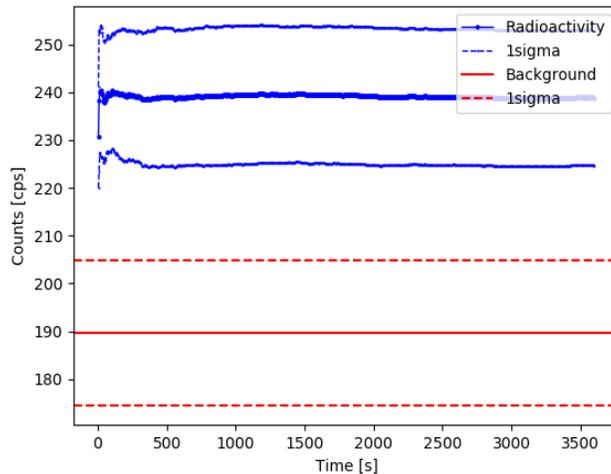
The integral count rate (600-1800 keV) shows a radioactivity over the background and generates an alarm in few seconds.
