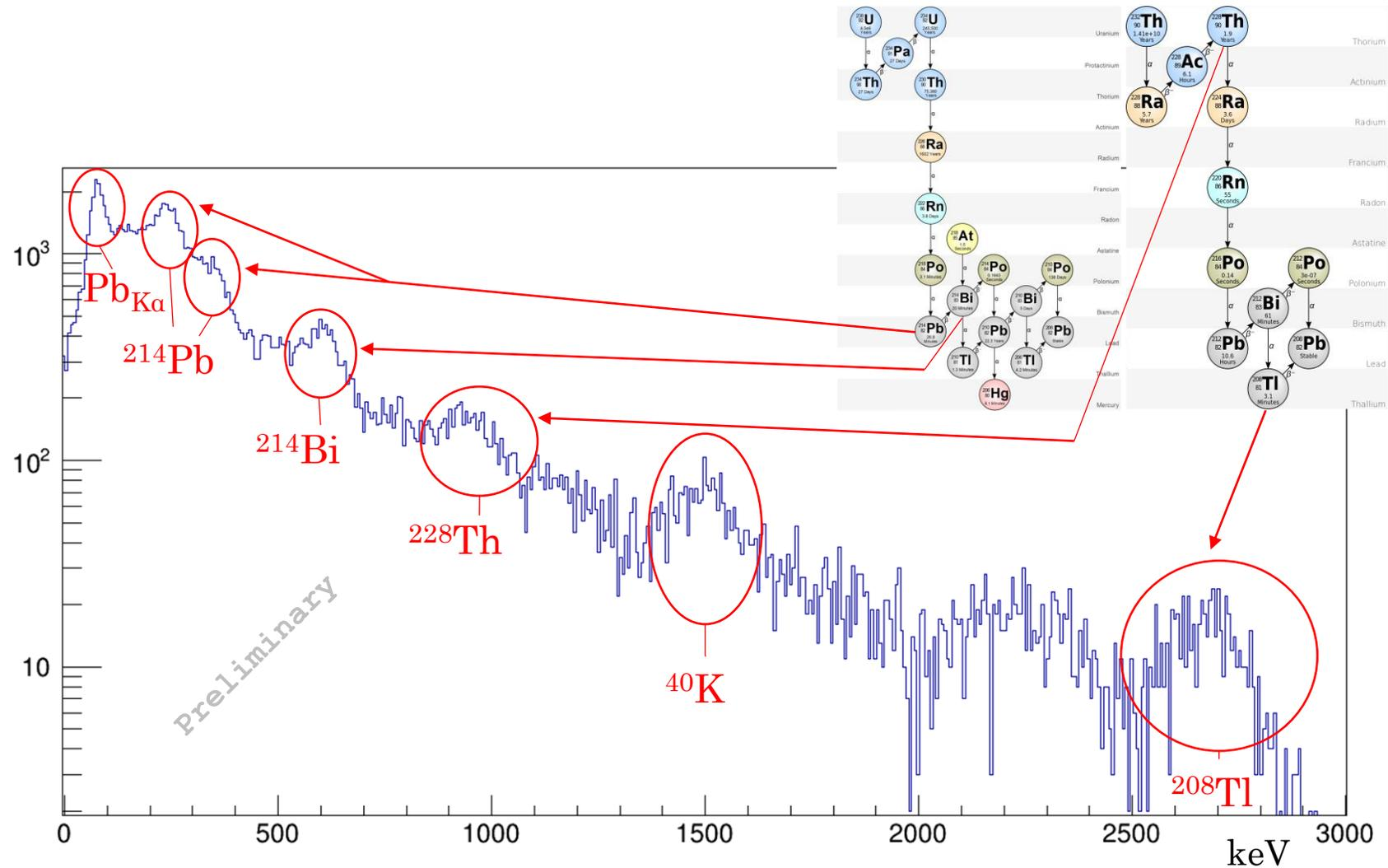
A NORM igneous rock was acquired with Camera to identify the main natural gamma radioactive peaks. The expected radionuclides was  $^{238}\text{U}$  and  $^{232}\text{Th}$  decay chains and  $^{40}\text{K}$ .
