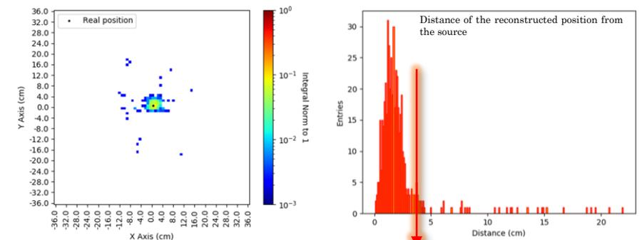
Black point show the real position of the source (random position normalized to center), the binned data the reconstructed positions. Data come from simulation.
