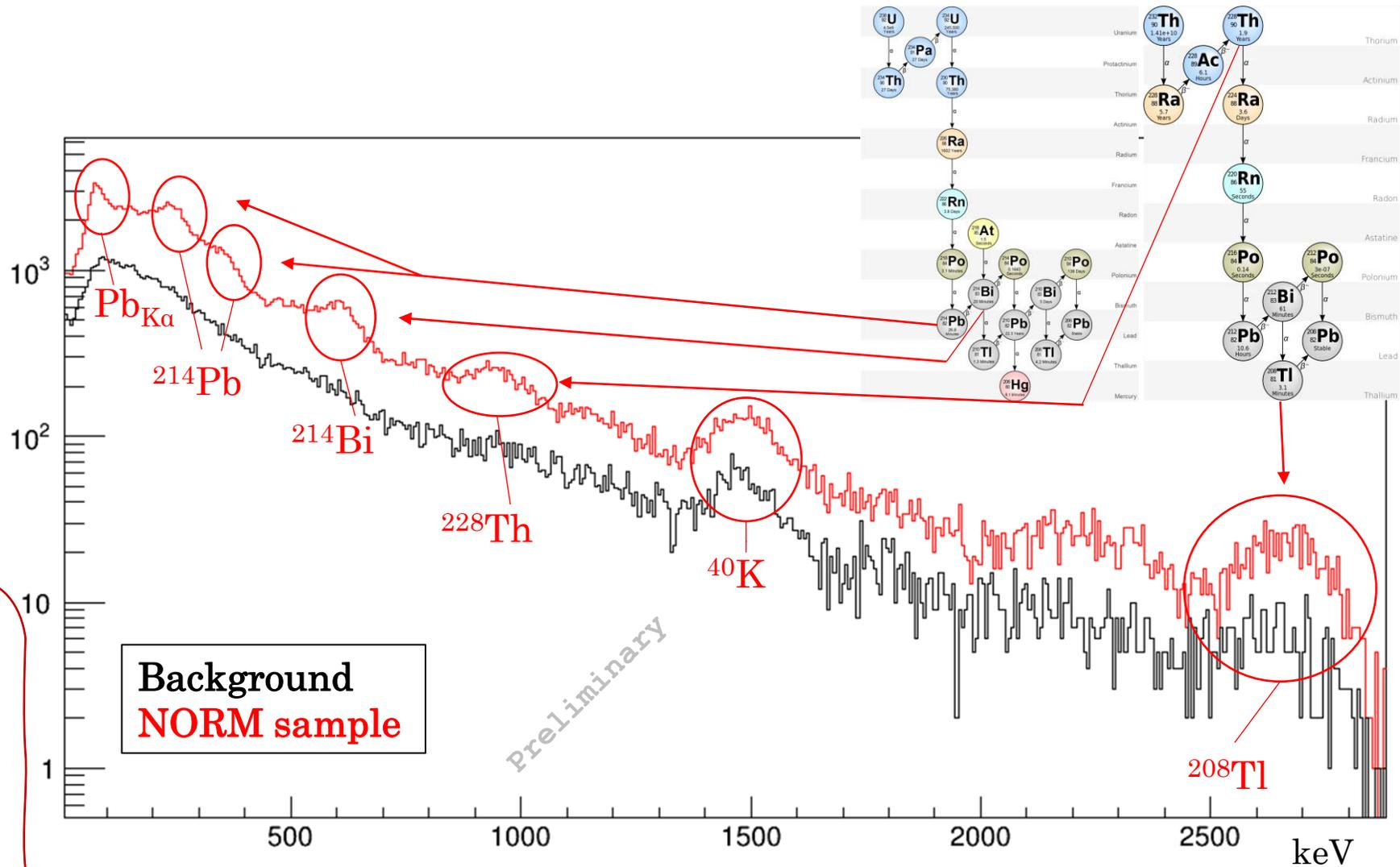
A NORM igneous rock gamma spectrum was acquired with Camera to identify the main natural gamma radioactive peaks. The expected radionuclides was  $^{238}\text{U}$  and  $^{232}\text{Th}$  decay chains and  $^{40}\text{K}$ .
