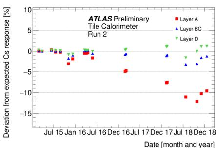
Fig. 3- Deviation of the average cell response to the Cs,  $\Delta R_{Cs}$ , (left) and to the Laser,  $\Delta R_{Las}$ , (right) during the Run 2 [2].
