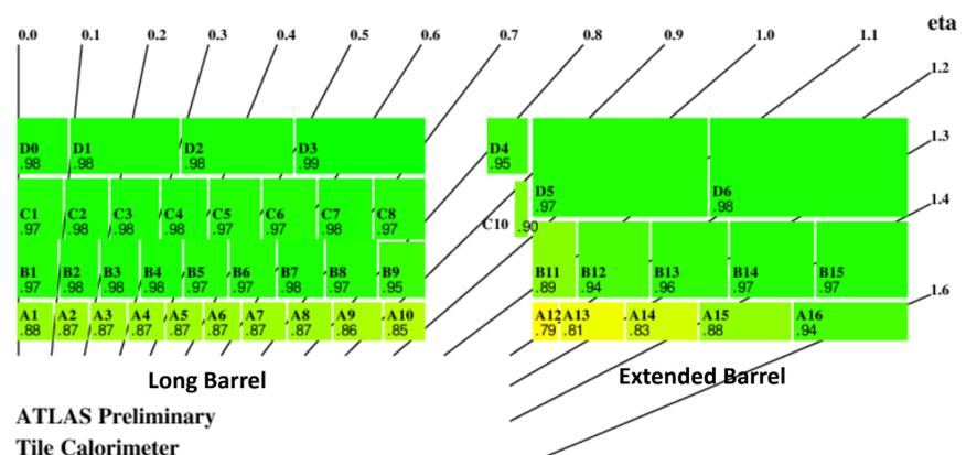
Fig. 7- Expected  $I/I_0$  of the TileCal cells in the end of Run 3. The relative uncertainty on the extrapolation ranges from 8 to 16% for cells in the A layer, in the Extended Barrel B layer, and the C10 cell, and is around 5% for the remaining cells [2].
