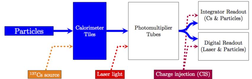
Fig. 2- Schematic of the TileCal Calibration Systems [2].
