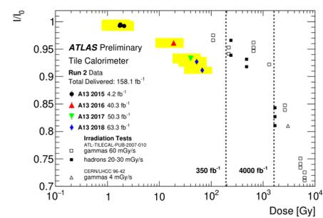
Fig. 4- Measured  $I/I_0$  for the A13 cell as a function of the simulated dose. The vertical errors are associated to the precision of the Cs ( $\sim 0.3\%$ ) and the Laser ( $\sim 0.5\%$ ) systems, and the horizontal error correspond to the dose spread within the large cell volume. The points with no error bars illustrate the laboratory measurements done on bare optical components (tiles or fibers) prior to the calorimeter construction [2].
