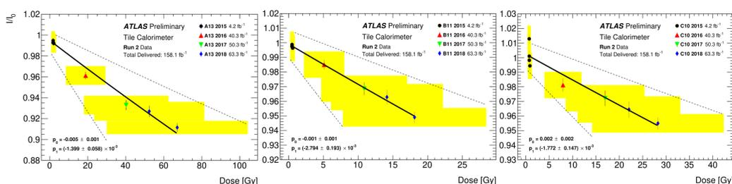
Fig. 6-  $I/I_0$  for the A13 (left), B11 (center) and C10 (right) cell as a function of the simulated dose during the LHC Run 2. The black solid line is the exponential fit, with the dashed black line corresponding to the exponential fit to the up and down uncertainty variations [2].
