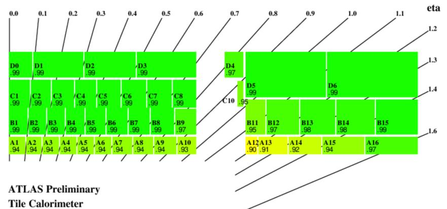
Fig. 5- Measured  $I/I_0$  of the TileCal cells in the end of Run 2. The relative uncertainty is of the order of 1%. Measurement in the D layer are not yet sensitive to a light yield degradation [2].
