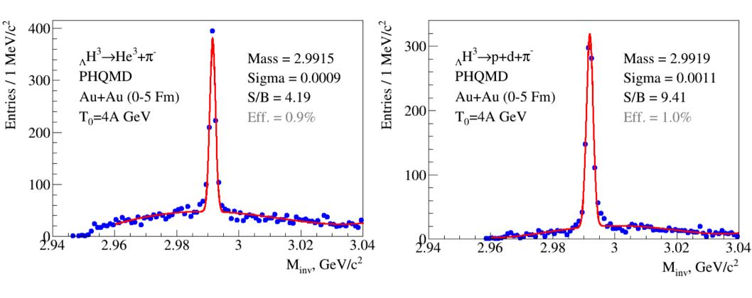
Reconstructed invariant mass spectra of  $_{\Lambda}H^3$ : 2-prong and 3-prong decay modes. Narrow peaks with  $\sigma$  of the Gaussian fit about 1 MeV/c² with quite high significance and signal-to-background ratio.
