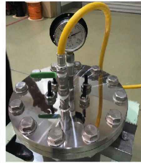
Underwater electronics: Case design and feedthrough
