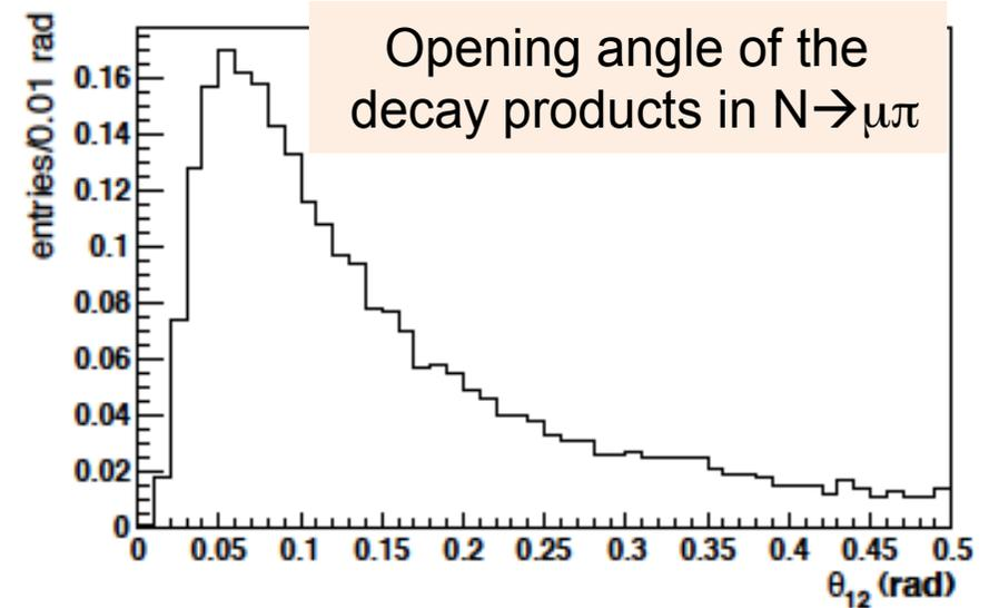
*Detector must be placed close to the target to maximize geometrical acceptance
