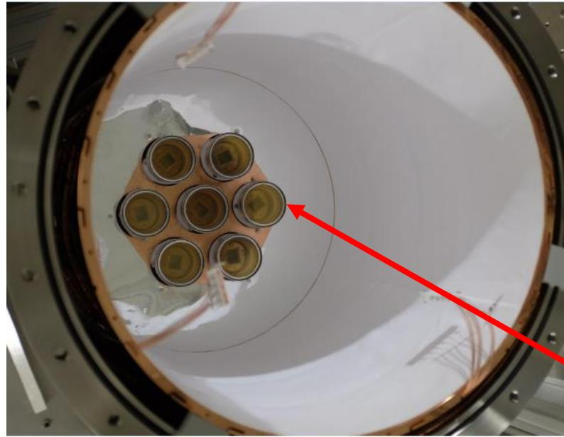
LAr scintillation veto works in the coincidence with Ge detectors allowing to suppress background events which deposit energy in LAr.
