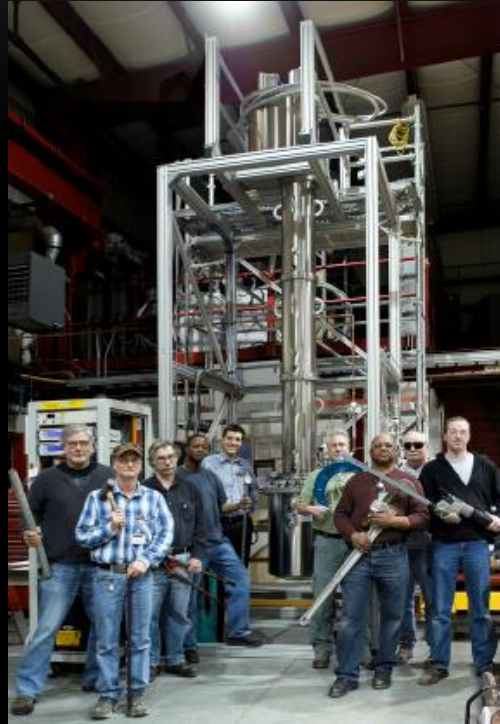
Distillation at Fermilab Separate Ar from N 2 / He
