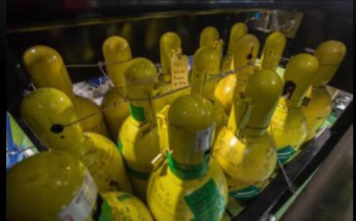
UAr bottles (156 kg) at LNGS Final purification with getters
