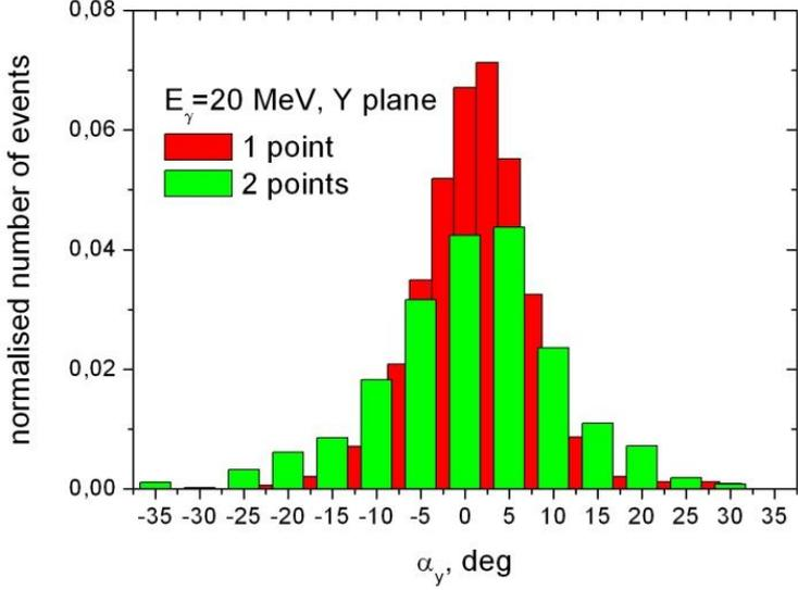
The distributions for the space deviation angle between restored and initial directions
