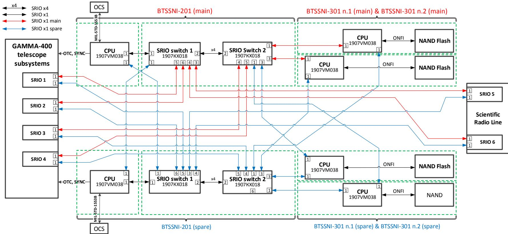
The total number of SDAQ operating configurations with BTSSNI-001 main and spare modules is 32
