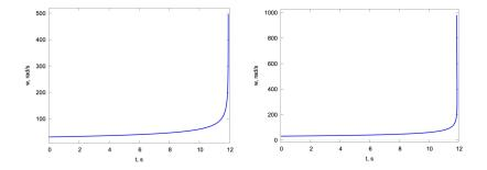
Figure: Graphs for  $\omega(t)$  for (a) Runge-Kutta method and (6) perturbation theory method
