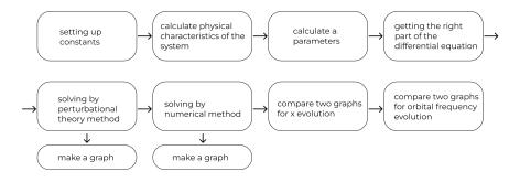
Figure: the way code on maxima works
