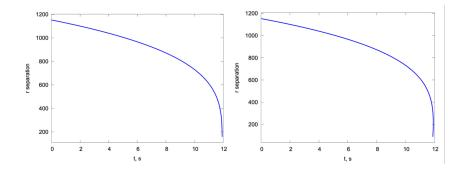
Figure: Graphs for  $r_{sep}(t)$  for (a) Runge-Kutta method and (6) perturbation theory method
