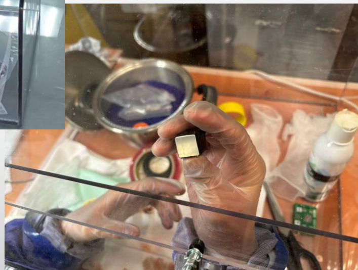
Polishing and wrapping crystal in Teflon tape
