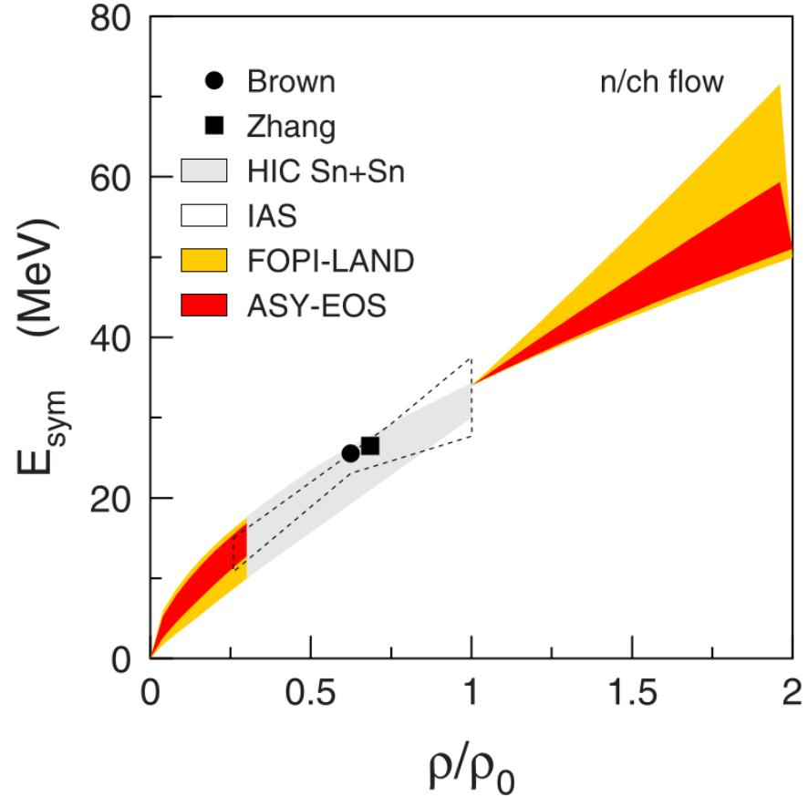
FIG. 18. Constraints deduced for the density dependence of the symmetry energy from the present data in comparison with the FOPI-LAND result of Ref. [5] as a function of the reduced density  $\rho/\rho_0$ . The low-density results of Refs. [78–81] as reported in Ref. [82] are given by the symbols, the gray area (HIC), and the dashed contour (IAS). For clarity, the FOPI-LAND and ASY-EOS results are not displayed in the interval  $0.3 < \rho/\rho_0 < 1.0$ .
