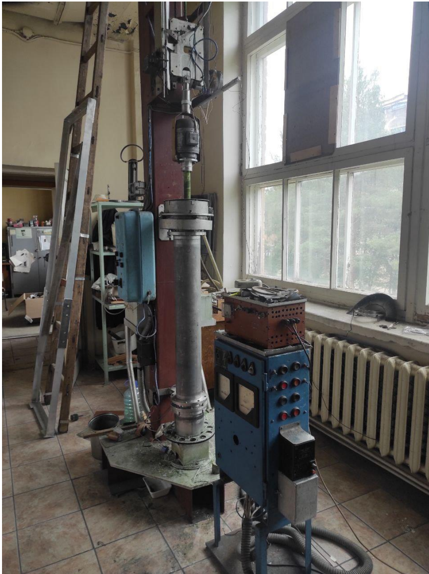
Pipe final polishing machine
